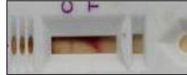
**Red staining obscures** the area where the test line should be. Control line is visible, but it is **unclear whether the test line is present or absent**.
